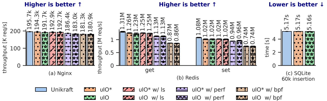
Figure 9: Application performance under uIO. uIO* is no MPK isolation. (a) Nginx throughput with wrk. (b) Redis throughput with redis-benchmark. (c) SQLite insertion time for 60k rows. “w/ ls” and “w/ perf” means we run the commands in the uIO every second. “w/ bpf” means we attach an eBPF program to some of the function calls to count the number of calls.
