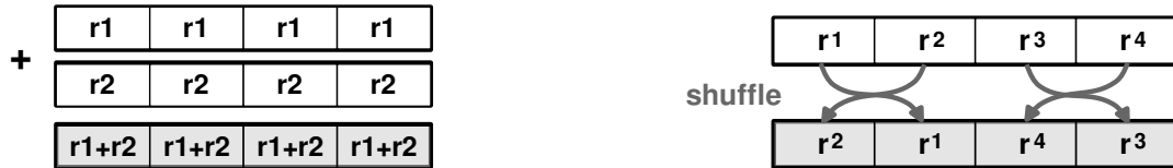
Figure 4.3 – AVX addition (left): original values r1 and r2 are replicated throughout the AVX registers; AVX shuffle (right): original values are rearranged.
