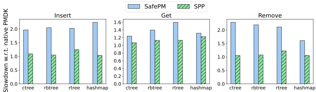
Figure 3.11: Performance overheads (throughput) of persistent indices for SPP and SAFEPM w.r.t. the native PMDK execution.
